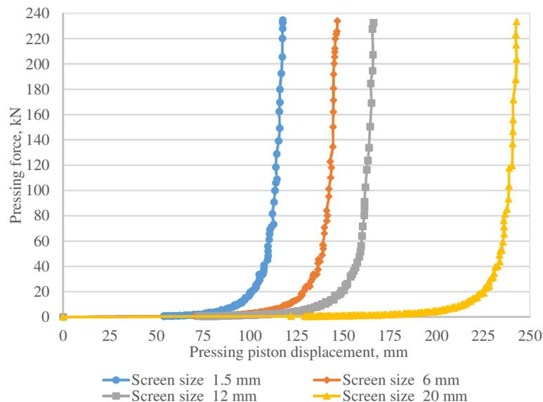
Fig. 4. Force – displacement characteristics of compacting
