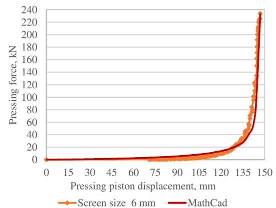
Fig. 6. Force – displacement (sieve 6 mm)
