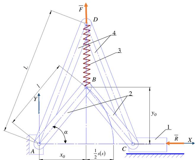
Fig. 3. **Rhomboid resistance mechanism model:** 1 – pressing piston; 2 – pressing links; 3 – spring element; 4 – supporting links
