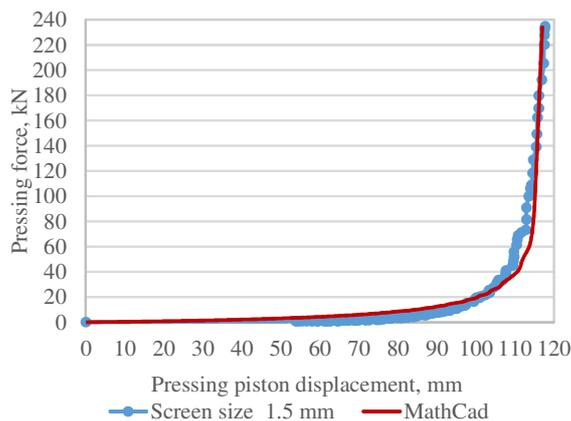
Fig. 5. Force – displacement (sieve 1.5 mm)
