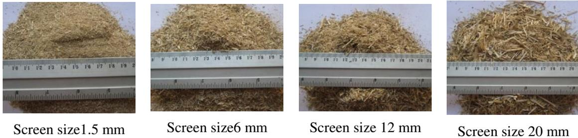
Fig. 1. Grinded common reeds
