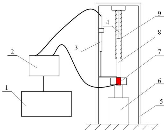
Fig. 2. **Compacting scheme:** 1 – computer; 2 – Pico Data Logger; 3 – displacement transducer; 4 – biomass; 5 – frame; 6 – hydraulic press; 7 – force measurement sensor; 8 – piston; 9 – cylindrical
