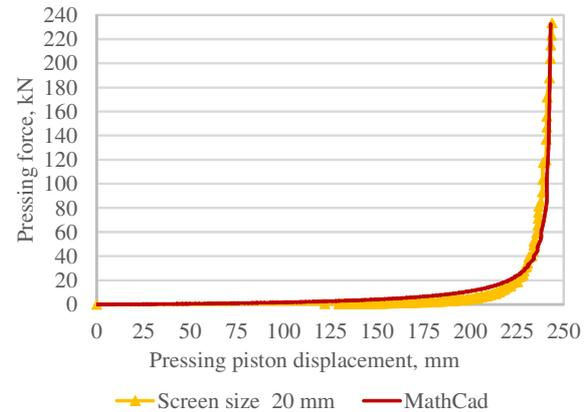
Fig. 8. Force – displacement (sieve 20 mm)
