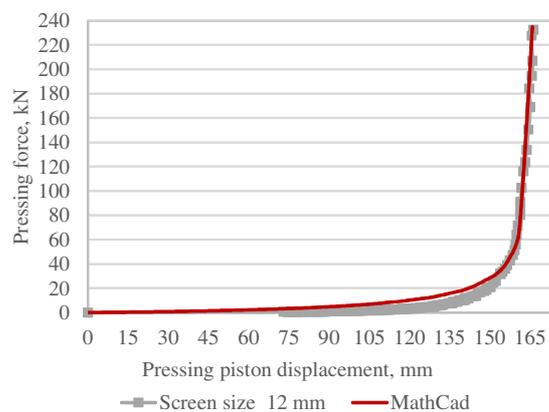
Fig. 7. Force – displacement (sieve 12 mm)
